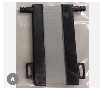
Figure 3. A) The coated SiC flat membrane, core of the AM-MF unit, B) Transmission electron microscopy (TEM) image of a SiO 2 nanosphere surrounded by TiO 2 active layer and C) TEM image of a ZnO nanoflower. The table lists some important requirements of the active nanoparticles for the AM-MF unit, in a comparison between SiO 2 @TiO 2 and ZnO.
